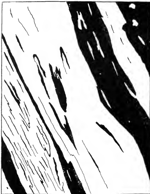
Fig. 36—Sixth level, Garson mine, Sudbury area, Ontario, showing manner in which the sulphides replace the schistose rocks. Width of face 3 feet. Black represents sulphides; white, rock.
